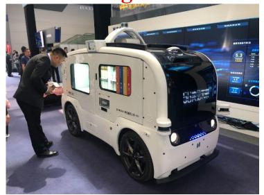
In Ziyang, Sichuan province, a logistics company has deployed three autonomous delivery vans as "employees." These driverless vehicles can transport 600 to 800 parcels continuously, navigating winding roads between villages 10 to 30 kilometers from their distribution center at speeds of 15 to 20 km/h. They stop at red lights, avoid obstacles, and are remotely monitored via smartphone.
