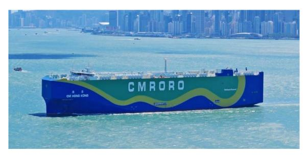
Hong Kong has taken a significant step toward sustainable shipping with the maiden voyage of the "CM HONG KONG," the world's first methanol dual-fuel roll-on/roll-off (RoRo) car carrier. Developed by China Merchants Group and named after Hong Kong, this vessel is the largest of its kind, capable of carrying up to 9,300 vehicles across 13 decks, including cars, buses, and heavy machinery.
